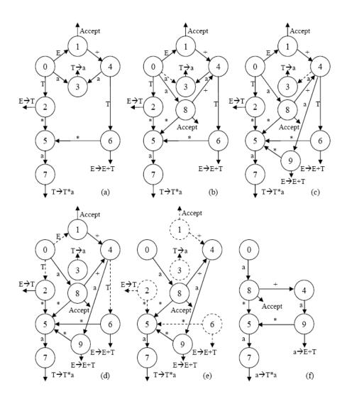
Fig. 2. Apply Unit Production Elimination on the LR(1) parsing machine of grammar G1
